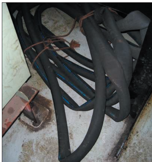
A flexible hose believed to have been used as the “magic pipe.” USCG photo
