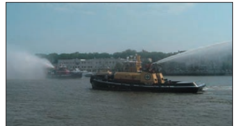
Moran and Crescent towing vessel operate FiFi Class I fire fighting systems. Each is capable of delivering more than 11,000 gallons of water per minute. USCG Photo
