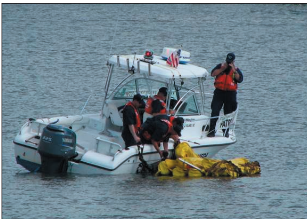
Members of the Coast Guard Auxiliary and MSU Savannah work to deploy oil containment boom delivered into the river by a Coast Guard helicopter. USCG photo
