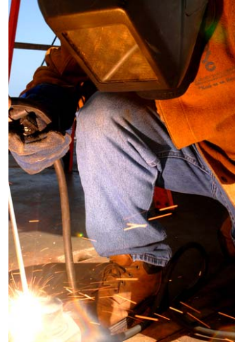
CARIBBEAN SEA - A NOAA technician welds the shackle that connects the chain to the anchor of the buoy before it is lowered 16,000 feet to the bottom of the ocean April 17, 2007. Coast Guard photograph by PA3 James P. Judge Jr.
